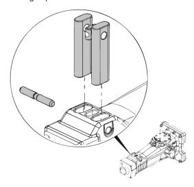
NOTICE The lock buffer in the tool retainer lock is made of plastic and can melt when operating in a hot environment. If this occurs, change the standard lock pin. Find optional spring pin in the spare parts list.
