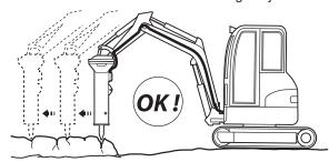
Never run the hydraulic breaker longer than 15 seconds on the same spot. Move the working tool to a new position if the object does not break.
