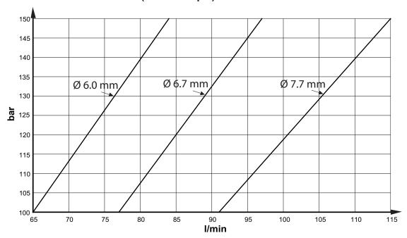
SB 552 Tunnel is delivered with restrictor  $\emptyset$ ??? for 110 bar (1595 psi) operation. As an option, restrictor  $\emptyset$ ??? for operation at higher pressure, is available.
