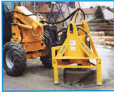
Kanaldeckelfräse Manhole cover cutter
